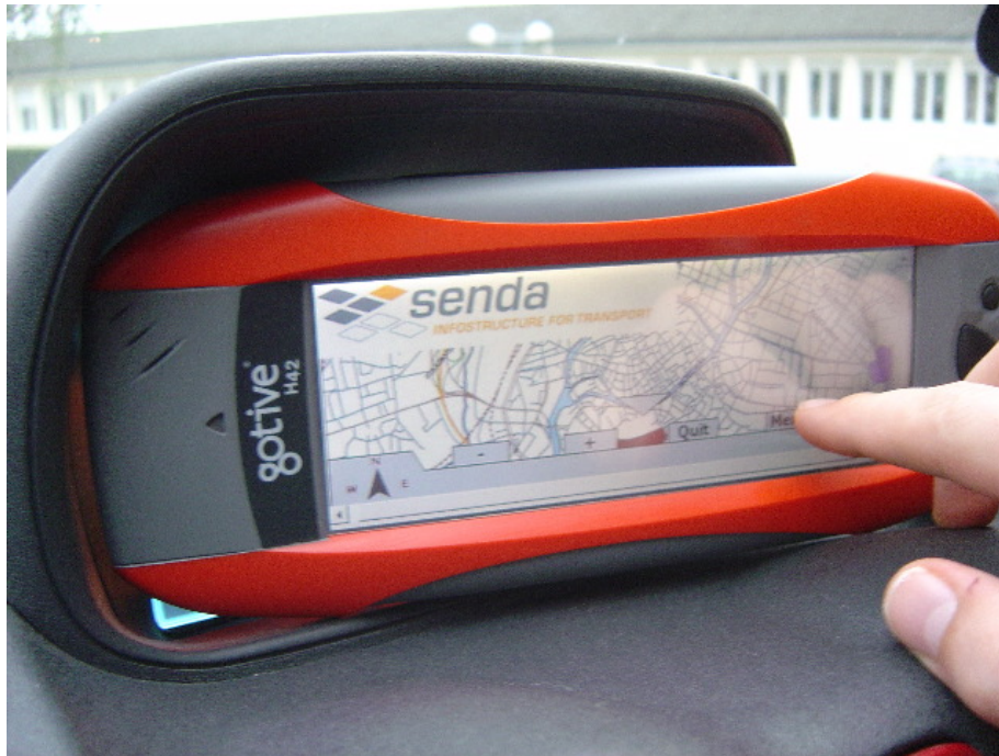
Figure 2: SENDA's Personal Navigation Device for Collaborative Navigation
