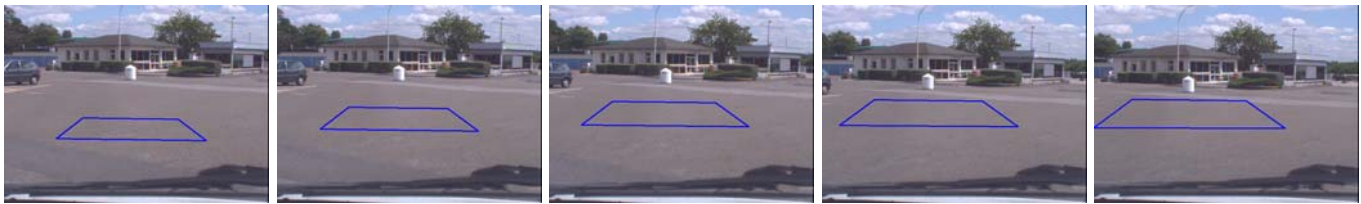
Fig. 9. An insufficient texture area (the patch is shifting)
