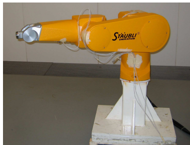
Figure 7: Flat configuration of a Stäubli Rx90
