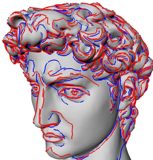
Figure 4: Crest ridges on the David. Red and blue lines distinguish crest associated to the maximal and minimal principal curvatures.
