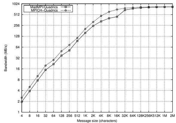
Figure 5. Raw point-to-point ping-pong - Bandwidth over Elan/Quadrics.
