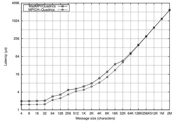
Figure 4. Raw point-to-point ping-pong - Latency over Elan/Quadrics.
