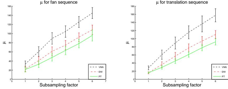
**Fig. 3.** Variation of error reconstruction relatively to sub-sampling factor with interpolation degree = 1. Left fan motion. Right translation motion. Three methods are evaluated : VNN, DW and PT. The PT method outperforms others methods especially on sparse data.
