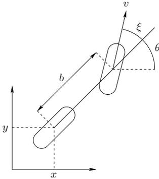
Fig. 2. The car-like vehicle  $\mathcal{A}$  (bicycle model).
