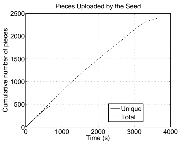
Figure 8: Number of pieces uploaded by the seed (limited to 200 kB/s), for a single representative run. The Unique line represents the pieces that had not been previously uploaded, while the Total line represents the total number of pieces uploaded so far. We observe a 14% duplicate piece overhead.
