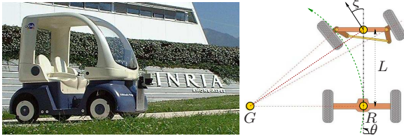
Fig. 5. The Cycab vehicle and its kinematics.
