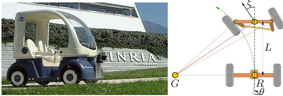
Fig. 5. The Cycab vehicle and its kinematics.
