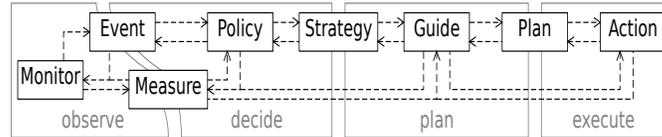
Figure 3: Detailed architecture of the DYNACO framework: entities and dependencies belonging to each FRAC TAL component.
