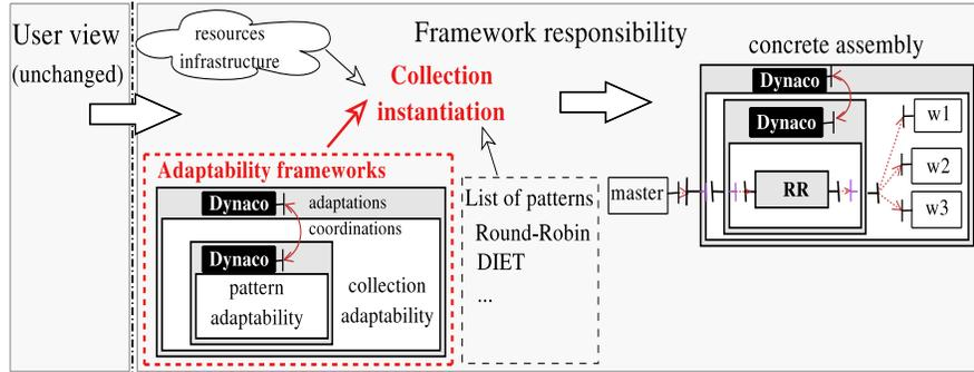
Figure 5: Introducing dynamic management in the *master-worker* model.
