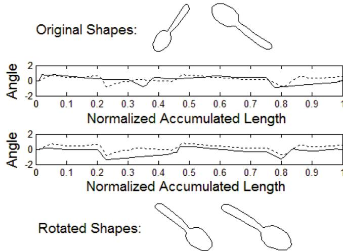
**Fig. 1.** Shapes and arc-length plots before and after the fitting process. A normalized cross correlation is computed between the two functions to determine the shift between them, thus normalizing the shapes to a certain rotation.
