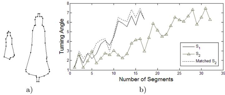
**Fig. 2.** Angle fitting. (a)  $S_1$  and  $S_2$ . (b) Turning angle plots. The influence of the number of segments composing the shape has been avoided, and the resulting turning angle plots are comparable.
