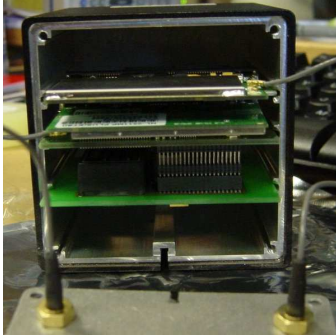
Figure 7. A 4G cube has two MiniPCI slots and two antenna sockets which are used to install two Wi-Fi cards. One is a 802.11b used for the VANET (to achieve longer communication ranges), while the other optional one can run in G mode to provide in-car wireless connections.
