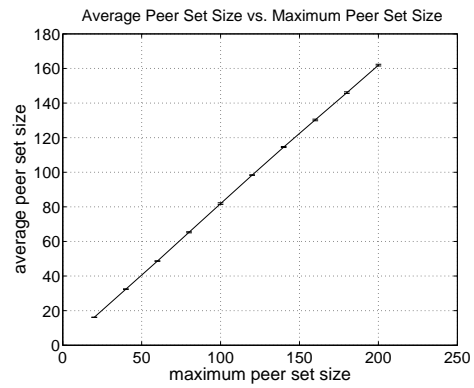
Fig. 14. The average peer set size as a function of the maximum peer set size, averaged over ten independent runs. The error bars indicate the minimum and maximum. The average peer set size is a linear function of the maximum peer set size.
