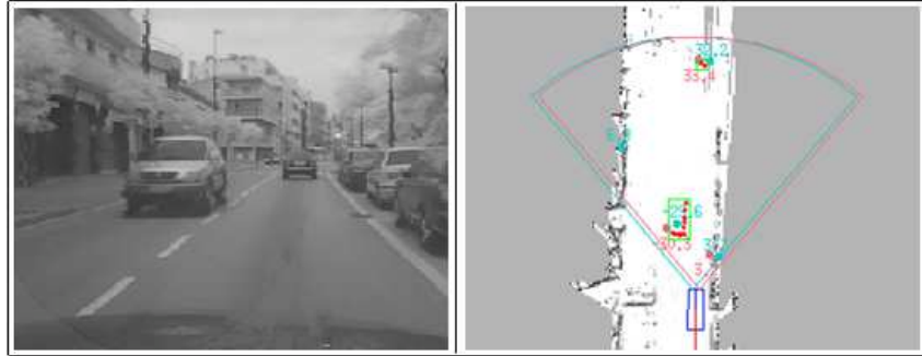
Figure 8: Moving object detected from laser data is confirmed by radar data.
