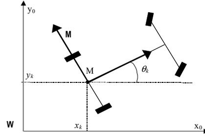
Figure 2: The mobile frame attached to the car
