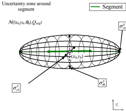
**Figure 4: Ellipsoidal of probability construction representing zone around a segment for horizontal segment i.e. parallel with the east axes**
