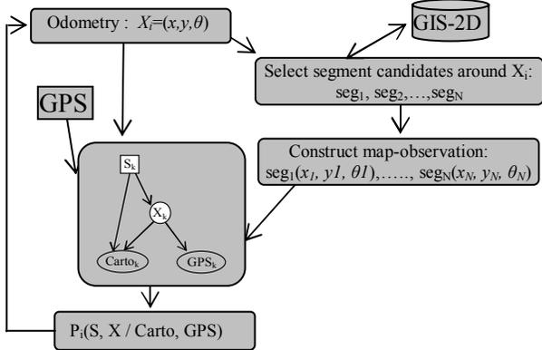
**Figure 7: Synoptic of road-matching using a BN**
