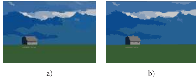
Figure 10: Ordering the feature spaces. Results of the balloon mean shift partitioning on the outdoor image when the feature spaces are ordered in the following ways: a) x-coordinate, y-coordinate, red channel, green channel, blue channel; b) blue channel, green channel, red channel, y-coordinate, x-coordinate.
