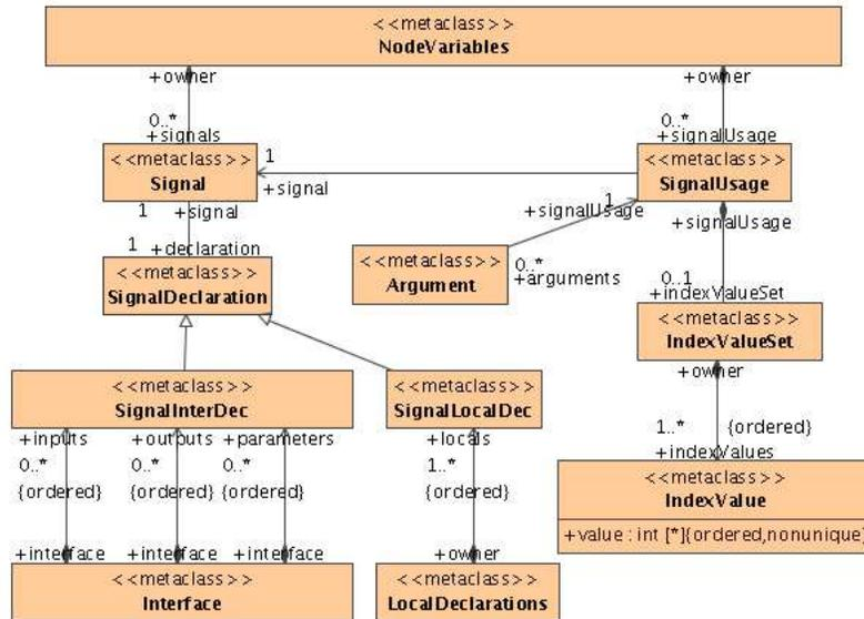
Figure 5: Extract of the synchronous metamodel: **Signal**.
