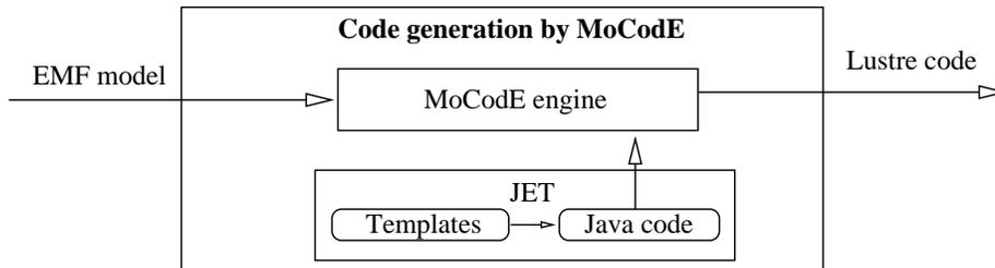
Figure 14: Generation of synchronous code from synchronous models.
