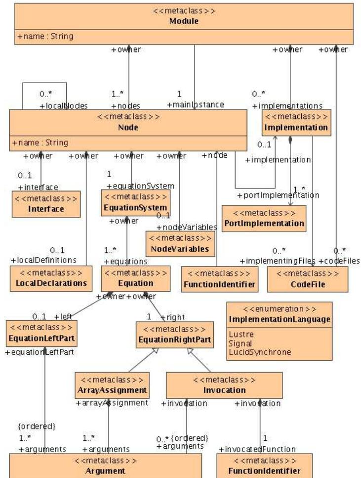
Figure 6: Extract of the synchronous metamodel: Node, Equation.
