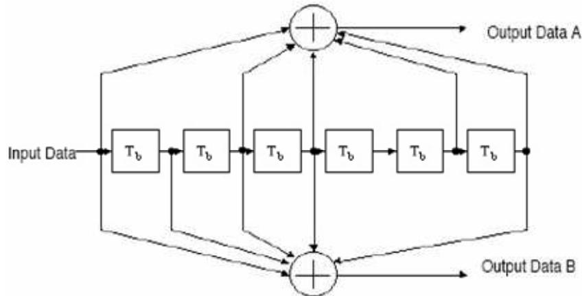
Figure 2. The Convolutional Encoder Used in IEEE 802.11a (from [18])
