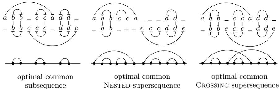
**Fig. 1.** Comparison of the optimal common subsequence and the optimal common supersequences. The optimal common subsequence is derived from  $u$  and  $v$  with two arc-removings. The optimal common NESTED supersequence requires four arc-removings. In this example, it is necessary to allow crossing arcs in the supersequence to get the same cost as for the subsequence (third scheme).
