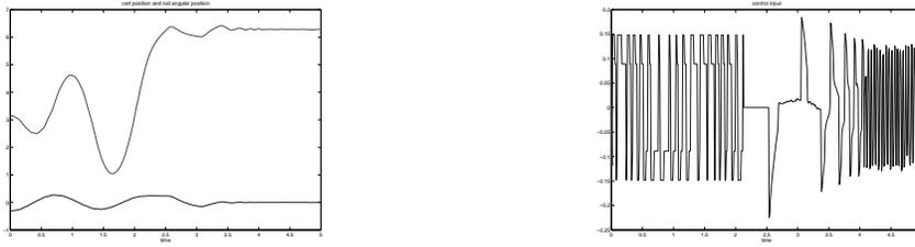
Figure 2: Experimental results: left cart and pendulum position, right control input.
