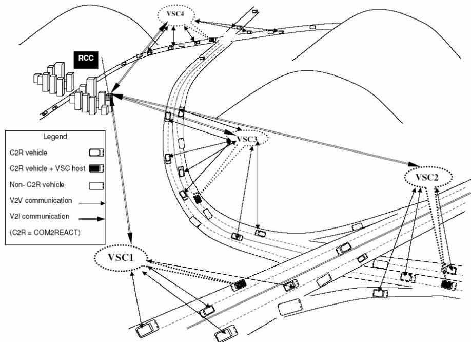
**Figure 1 The COM2REACT system and VSC concept**
