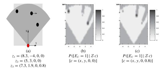
Fig. 2. Example of static grid estimation. (a) The situation and the sensor observations, given in  $(x, y, \dot{x}, \dot{y})$ . (b), (c) Values of occupancy probability for two "slices" of the four-dimensional grid, i.e., for all possible positions at a given speed.
