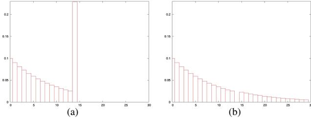
Fig. 2. (a) (resp. (b) ) shape of probability distribution over the possible sensor range measurements knowing that the 14th cell is occupied (resp. empty) including an error model and *a priori* over the occupancy of cells.
