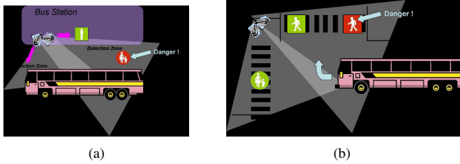
Fig. 1. (a) The bus arrives or leaves its bus stop. The vulnerables situated in the blind spot near the bus are in danger because they are not seen by the driver and have a good probability to enter in collision with the bus; (b) The pedestrian crosses at an intersection when the bus turns right.
