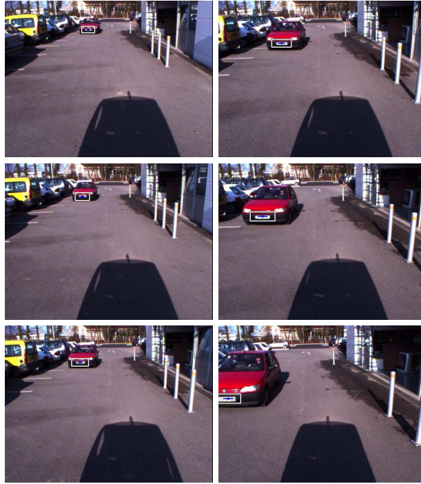
Fig. 4. Test sequence for ridge tracking : the licence plate of the car is tracked with our method. The rectangle represents the region of interest and the segment at center represents the position and the direction of the tracked ridge
