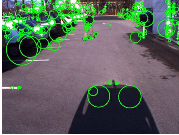
Fig. 2. Interest point detection. The size of the circles correspond to the intrinsic scale. Circular objects as the walker's body are well detected whereas stretched objects give unstable results.
