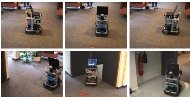
Fig. 10. The robot reach a last crossing. Ten red tokens are detected. The last behaviour is activated, and the robot enter the home.
