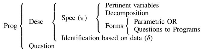
Fig. 1. Structure of a Bayesian Robotic Program.
