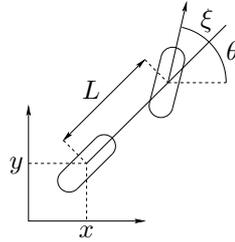
Figure 3: The car-like vehicle  $\mathcal{A}$  (bicycle model).
