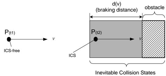
Figure 1: Inevitable Collision State vs. Safe State
