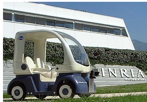
Fig. 10. the cycab: an autonomous car-like robot platform
