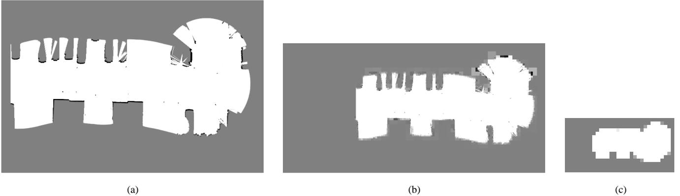
Fig. 8. Maps of the car park of INRIA. (a) The *OG* model contains 393,126 cells, while the *WOG* model contains 78,742 cells. (b) The *OG* model reconstructed from the previous *WOG* model; it can be seen that significant details such as beacons have been captured by the *WOG* representation (the shapes of maps (a) and (b) are very close). (c) The empty space is pretty well approximated at the coarser scale.
