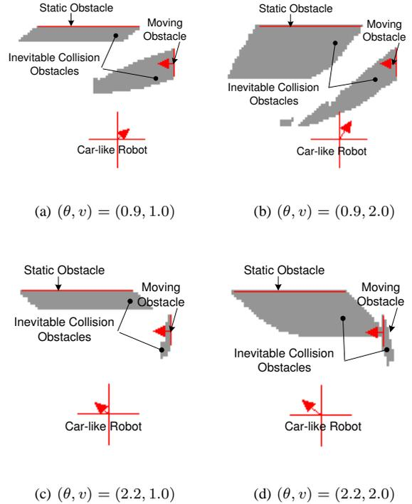
Fig. 12.  $(\theta, v)$ -slices of the state space of  $\mathcal{A}$ . Shaded regions are ICS respectively defined for the braking trajectory of control  $(\alpha_{min}, \dot{\xi}_{min})$  (top), and all braking trajectories with controls selected from  $[(\alpha_{min}, \dot{\xi}_{max}), (\alpha_{min}, 0), (\alpha_{min}, \dot{\xi}_{min})]$  (bottom).
