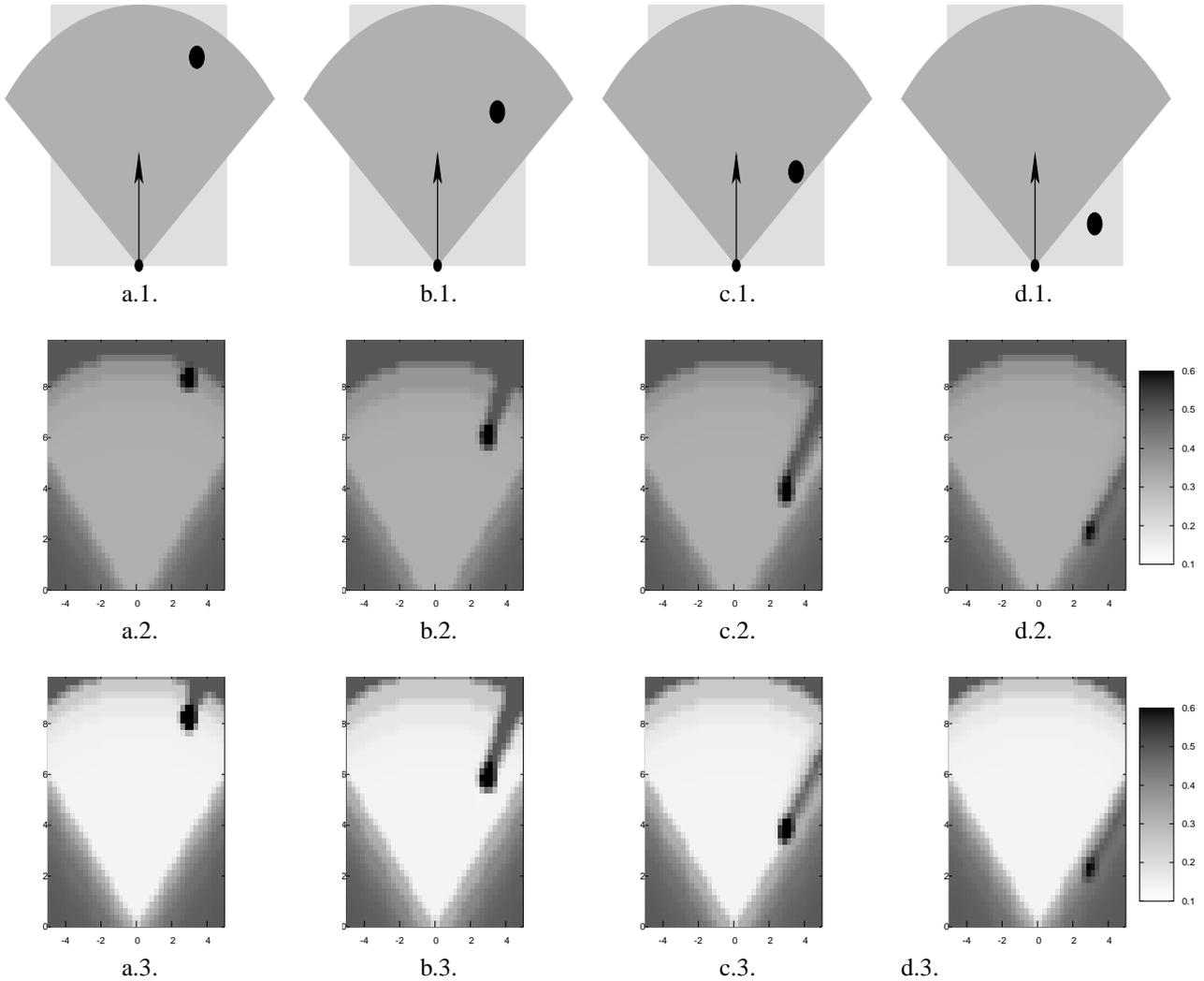
Fig. 4. A short sequence of a dynamic scene involving a stationary obstacle and the Cycab moving forward at a velocity of  $2.0 \text{ m/s}$ . The second and the third row respectively show the results of the prediction and of the estimation steps of the *BOF*, in a 2-dimensional slice of the grid corresponding to a relative speed of  $\dot{x} = -2.0$ , i.e.  $P([O_{x \ y}^t [\dot{x} = -2.0] [\dot{y} = 0.0] = occ])$ .
