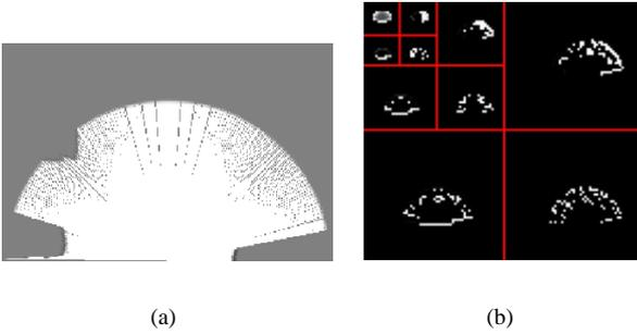
Fig. 6. Mapping obtained by a laser range-finder : (a) the obtained  $OG$  model; (b) the related three first ‘‘detail spaces’’ of the  $WOG$  model and the complementary scaled space. The density of non-zero coefficients decreases drastically in wavelet space.
