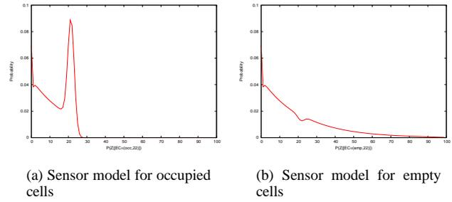
Fig. 1. Example of one-dimensional sensor models. The sensor is a laser-range finder located in  $x = 0$  and detecting an object at  $x = 22$ . The following property holds :  $P(Z|[O_x = occ]) = P(Z|[O_x = emp])$  for  $x > z$ , which implies that  $P(O_x|Z)$  is unknown when the cell is behind the obstacle.
