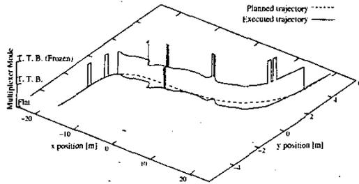
Fig. 12. Executed trajectory with respect to planned trajectory, and multiplexer mode.
