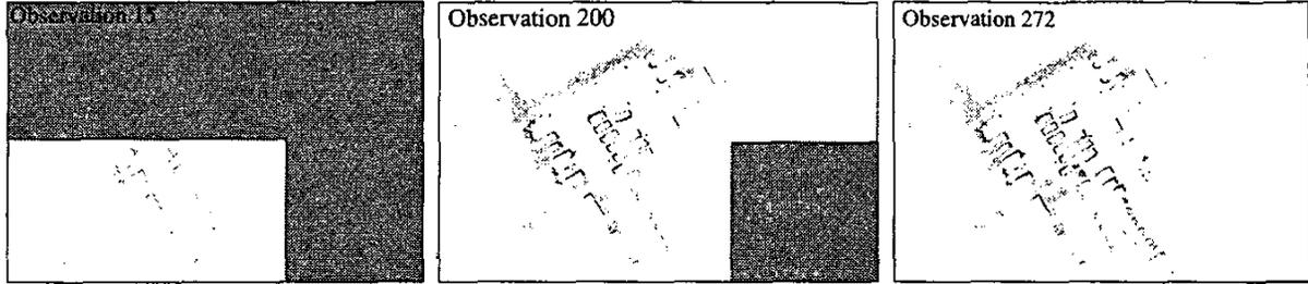
Fig. 2. Obstacle map evolution: Experimental map of the car-park area built during the obstacle map-building phase.
