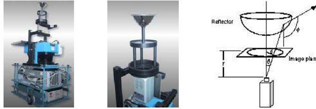
Fig. 8. System used for the experimentation: The fully autonomous robot Donald Duck and the panoramic vision system. The camera has a 640 \times 480 pixel resolution and an equiangular mirror is used so that each pixel in the image covers the same view angle.
