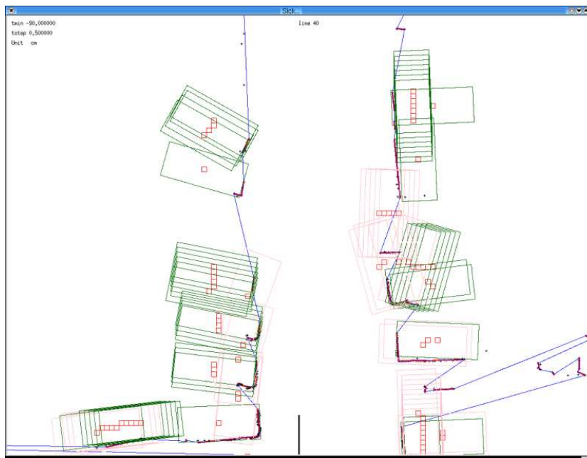
Figure 4.6: Filtering by the polygon of visibility. The polygon in blue indicates the polygon of visibility formed by segmentation. The green vehicles indicate valid positions and the red indicate vehicles eliminated by the filtering.
