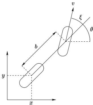
Fig. 9. The car-like vehicle  $\mathcal{A}$  (bicycle model).
