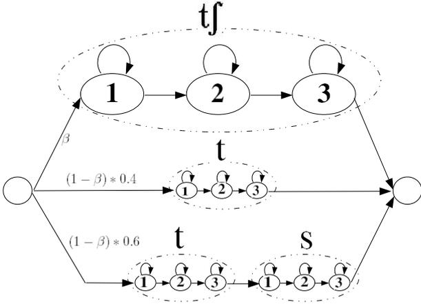
Figure 1: Adding HMM state paths to the model of the English phone [tʃ] in the case of Greek accent ( $\beta$  is a weight).
