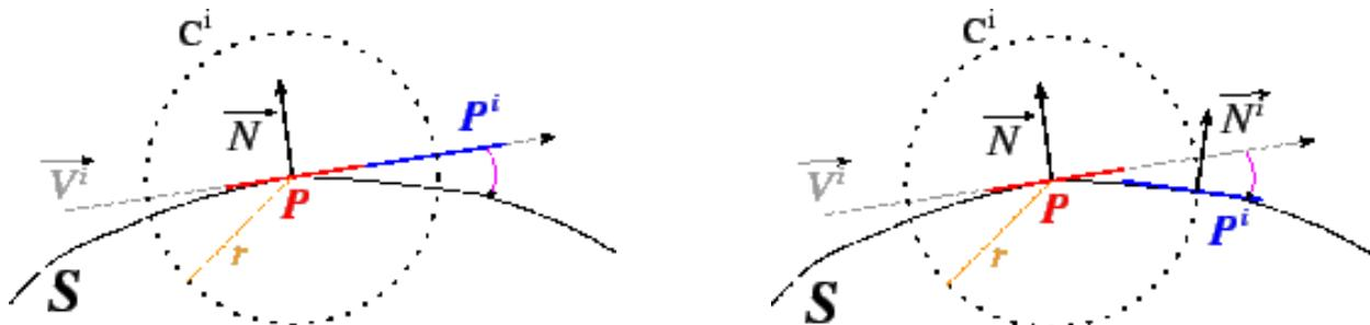
Figure 4 Re-projecting a particle on the surface. (left) Initial position of the child  $P^i$ . (right)  $P^i$  is reprojected according to circle  $C^i$ .
