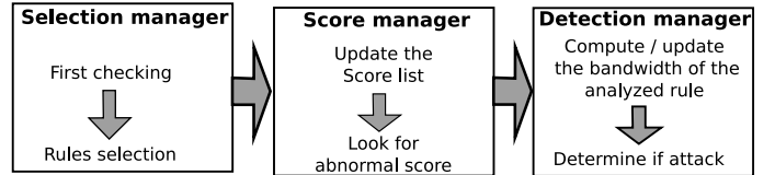
Fig. 2. The different components and the detection process
