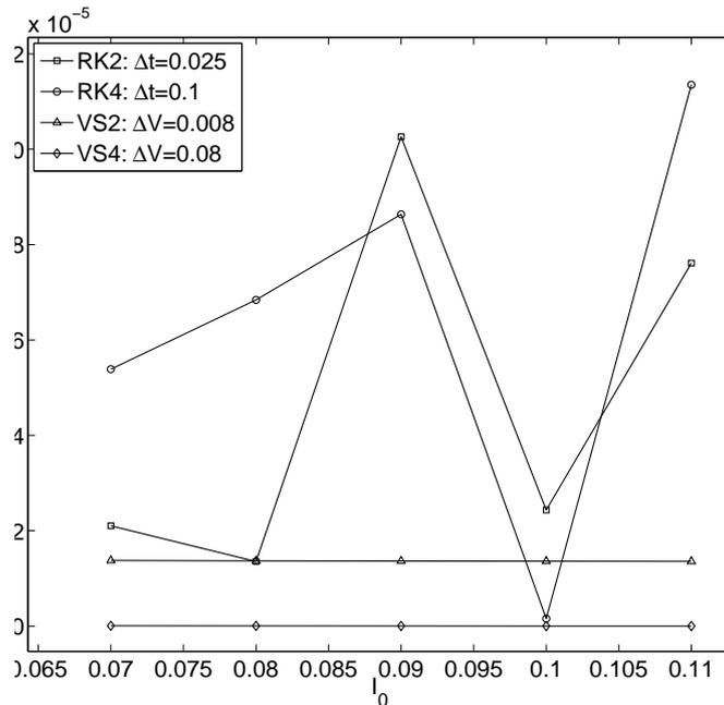
Figure 6: Error  $E(\nu)$  (in Hz) on the firing rate of the QIF neuron as a function of the input current. The squares and circles correspond to the modified RK2 with  $\Delta t = 0.025 ms$  and the modified RK4 with  $\Delta t = 0.1 ms$ , respectively. Triangles represent VS2 with  $\Delta v = 0.008$  and diamonds VS4 with  $\Delta v = 0.08$ .
