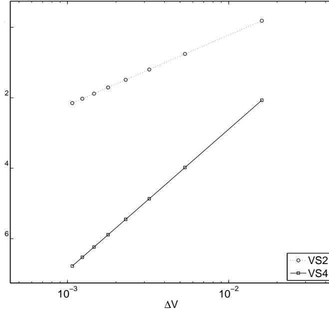
Figure 7: Log-Log plot of the error  $E(\nu)$  on the firing rate as a function of the voltage-step for the voltage-stepping methods VS2 (circle) and VS4 (square). The lines (not fits) indicate the order of the methods. Dotted-line is second order and solid-line is fourth order.
