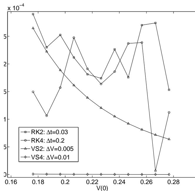
Figure 3: Error  $E(t^f)$  (in ms) on the firing time of the QIF neuron as a function of  $v(0)$  for different algorithms. Squares and circles are the modified RK2 with  $\Delta t = 0.03ms$  and RK4 with  $\Delta t = 0.2ms$ , triangles and diamonds are VS2 with  $\Delta v = 0.005$  and VS4 with  $\Delta v = 0.01$  respectively.
