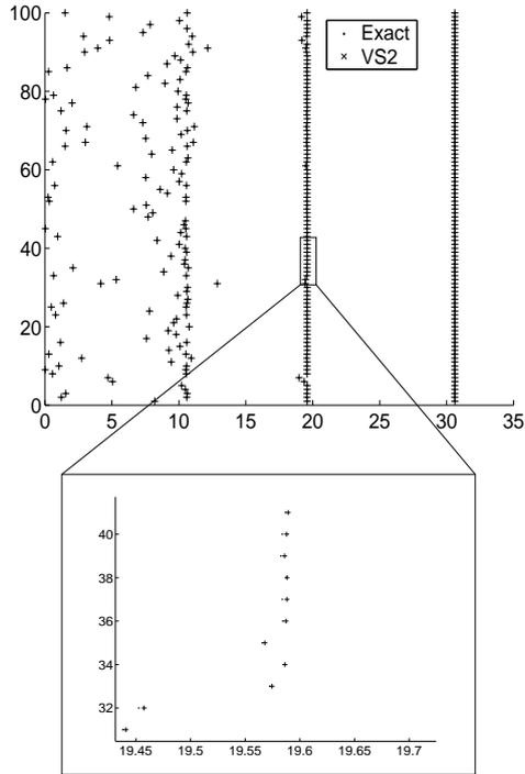
Figure 11: Simulation of a network of 100 inhibitory neurons. Spike times are computed exactly (dots) and with the VS2 method using  $N_{\Delta v} = 250$  voltage-intervals ('+'). A high degree of accuracy is obtained and spikes are superimposed most of time (see enlargement).
