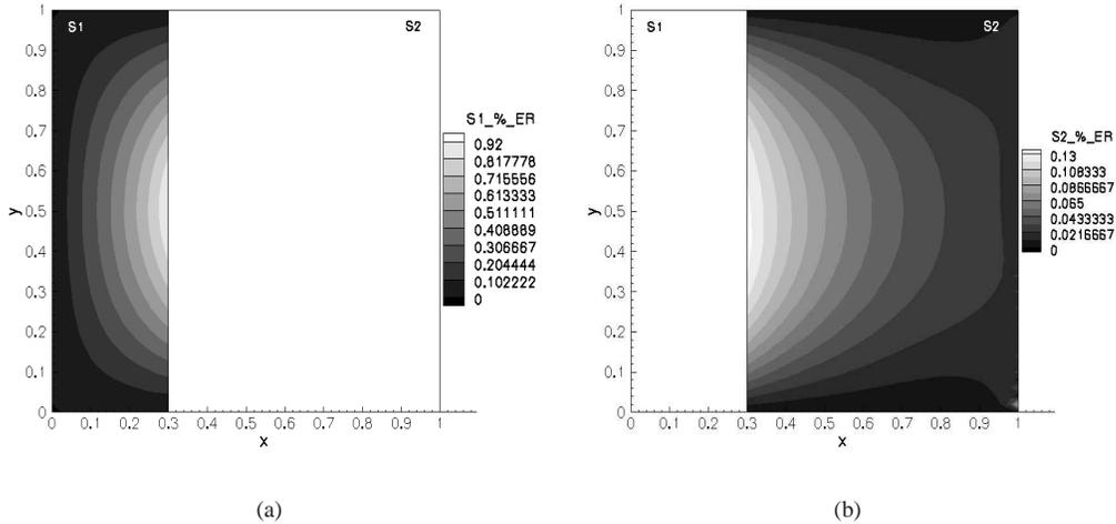
Figure 2: Distribution of the relative error between the solution obtained by the present method and the solution obtained by a second order FD method on the whole domain.  $\Omega_1$  (a),  $\Omega_2$  (b).
