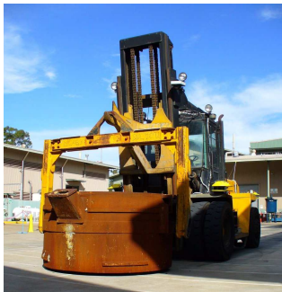
Fig. 1. Hot Metal Carrier picking up a crucible
