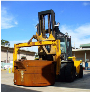
Fig. 1. Hot Metal Carrier picking up a crucible
