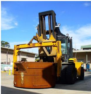
**Fig. 1.** Hot Metal Carrier picking up a crucible
