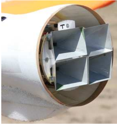
Fig. 3. The antenna configuration used within the UAV allows four individual radar units to monitor the flight path of the UAV for obstacles.
