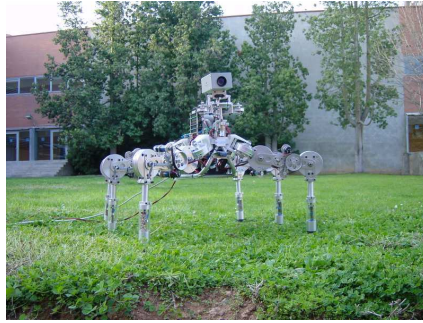
Fig. 2. The six-legged robot Lauron III used in the experiments.
