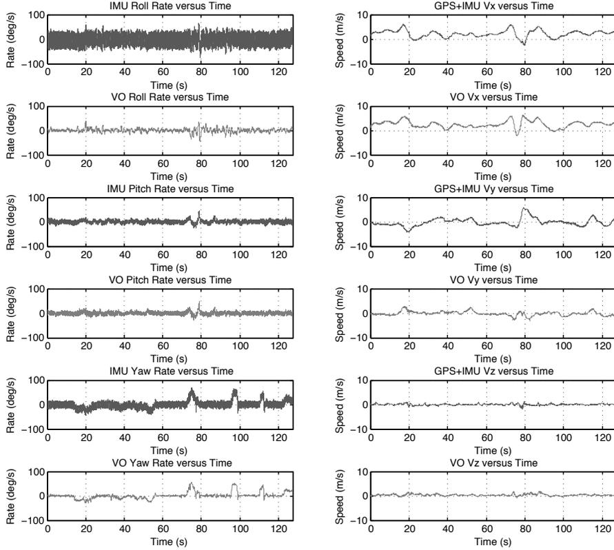
**Fig. 2.** Comparison of angular rates measured by the IMU and by VO (left column), and linear velocities measured by GPS+IMU and by VO (right column). All values are expressed in the helicopter body coordinate frame.
