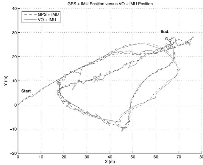
**Fig. 4.** Filtered GPS+IMU position estimate versus filtered VO+IMU position estimate. A single end label is shown, as the difference between the final GPS+IMU position and the final VO+IMU position is only 1.6 meters (after a 405.5 meter flight).
