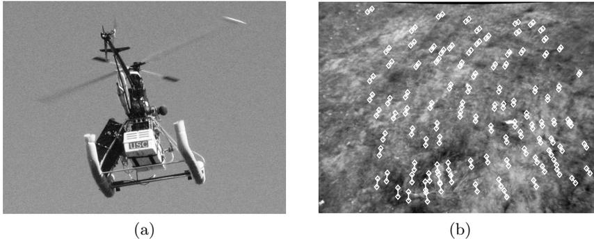
**Fig. 1.** (a) Helicopter during a data acquisition flight. The avionics box (white) is located beneath the main helicopter chassis; the vision computer (black) is mounted on left-hand side of the vehicle. Both stereo cameras are also visible near the front of the landing skids. (b) Two-frame feature tracks overlaid on a left stereo image.
