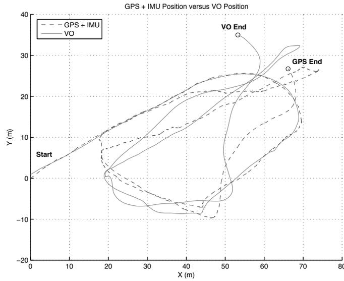
**Fig. 3.** Filtered GPS+IMU position estimate versus VO position estimate. The VO trajectory exhibits a characteristic misalignment due to the integration of small orientation errors over time. The difference between the final GPS+IMU position and the final VO position is 14.7 meters (after a 405.5 meter flight).
