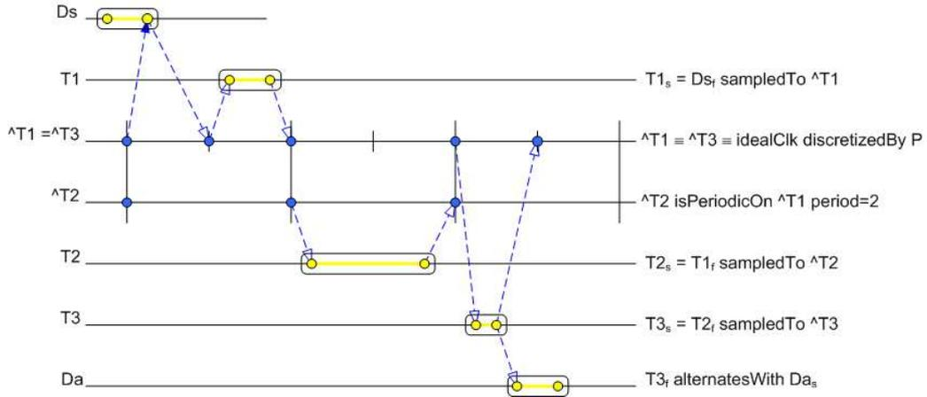
Figure 16. CCSL constraints, the harmonic down-sampling synchronous case.
