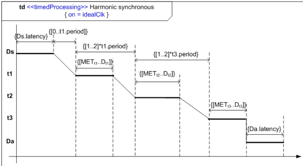
Figure 17. Timing diagrams, the harmonic synchronous case.
