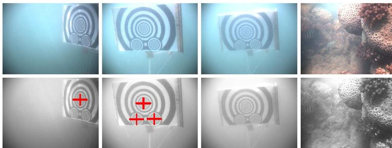
**Fig. 1.** SSL detection in marine environment. Upper row: original images, lower row: detection. From left to right: robustness to perspective and lighting discontinuity, minimum required contrast, insufficient contrast, absence of false positives in a natural environment.
