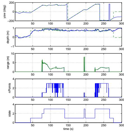
**Fig. 4.** AUV pose and SSL detection properties during a typical target identification and homing experiment. Here the AUV was required to identify the target and maintain a stand-off distance (range) of 2m.
