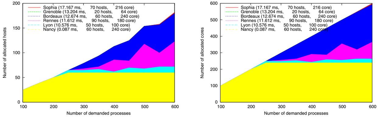
Figure 2. *concentrate* results: locations of allocated hosts (left) and allocated cores (right)
