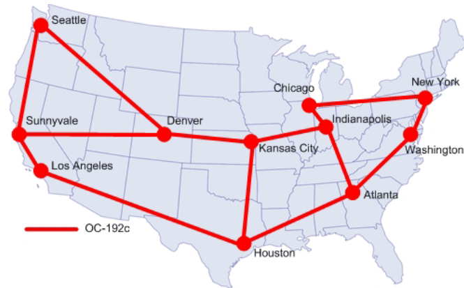
Figure 6: Abilene Network with 11 routers and 14 links.
