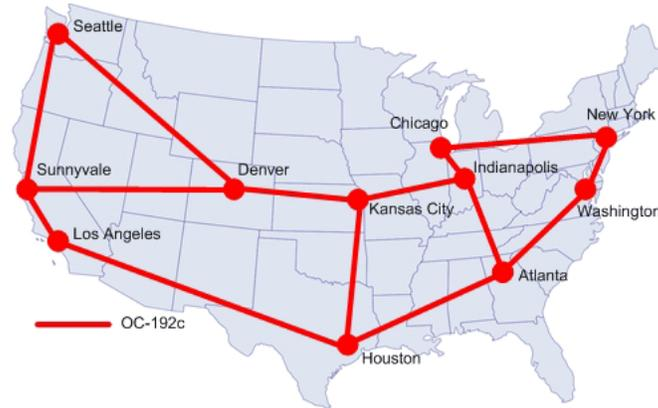
Figure 6: Abilene Network with 11 routers and 14 links.
