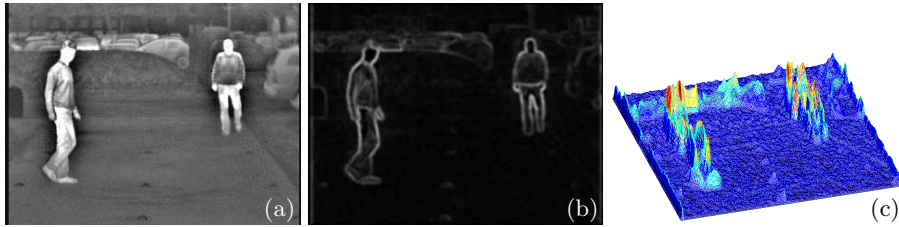
Fig. 3. Energy field due to edges: (a) original image, (b) edge image obtained using Sobel operator and gaussian smooth, (c) edge energy functional with inverted sign, to obtain a more effective graphical representation.
