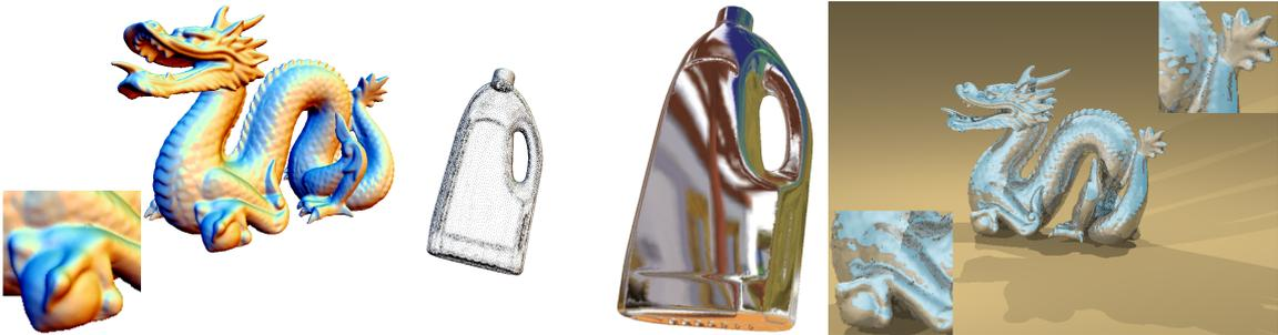
Figure 10: Different rendering of our surfaces. Left: Realtime rendering with OpenGL. Center: A raytraced image with a reflexion shader. Right: Direct use of *Cube Mapping* in OpenGL, an example of the immediate benefit of our technique.
