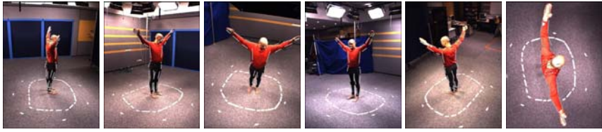
Fig. 5. A set of six calibrated cameras provides six image sequences whose frames are synchronized
