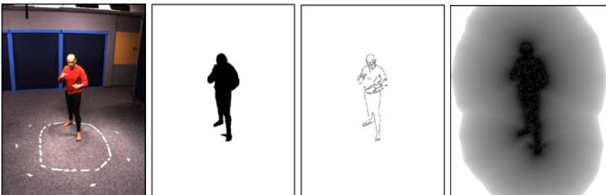
Fig. 4. From left to right: A raw image, the silhouette, the edges inside the silhouette, and the chamfer-distance image associated with the silhouette
